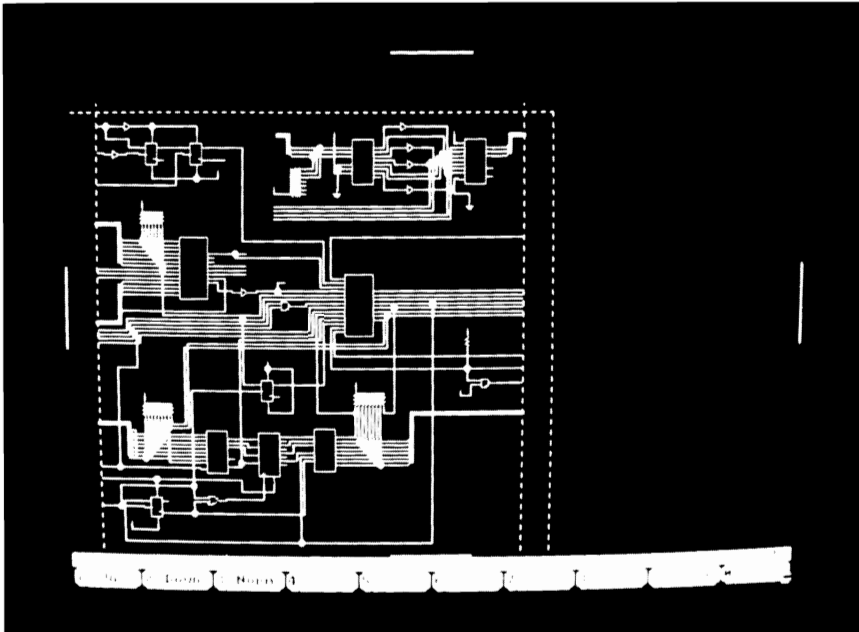
Fine detail is made possible in your schematics by the program's use of the high resolution interlaced mode
